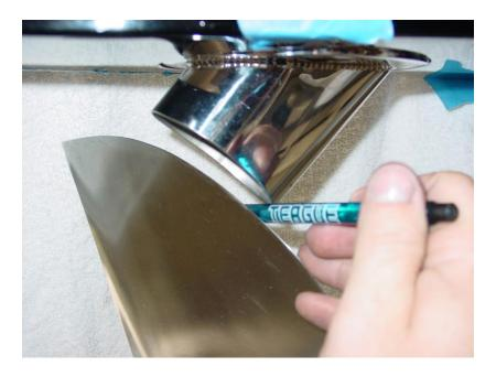
CAUTION! It is important that you maintain 1/4" to 3/8" clearance between the propeller and oval tube! Failure to do so will result in poor performance or damage to both the propeller and aerator assembly.
