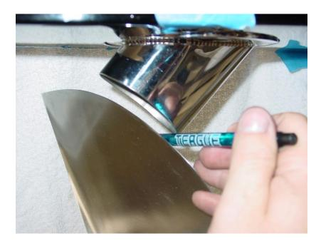
CAUTION! It is important that you maintain 3/8" clearance between the propeller and oval tube! Failure to do so will result in poor performance or damage to both the propeller and aerator assembly.
