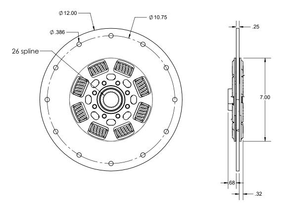
This will fit both 755-8602 top mount, neutral balanced steel flywheel as well as stock Mercury flywheel
